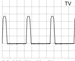
DC, 200V/Div, 20µs/Div T7583, Collector 53
