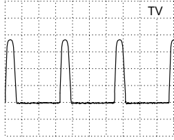
DC, 200V/Div, 20µs/Div T7583, Collector 53
